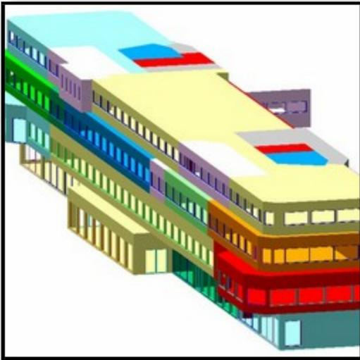
Computer generated 3D model of the building with colours denoting different zones
